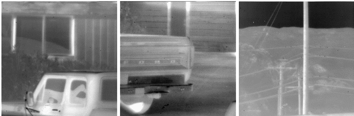
Figure 7. Images from the THPF mode test. When the THPF is running a slow update rate, very few image artifacts exist.
