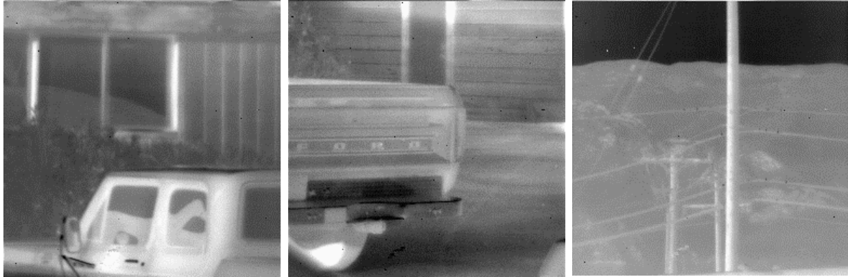
Figure 9. Images from the AIRS device running in “Temporal High Pass Filter” (THPF) mode. When the THPF is running at a slow update rate, very few image artifacts exist (images courtesy of Raytheon Infrared Operations).
